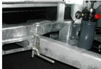
A Frame Clamp Loose
