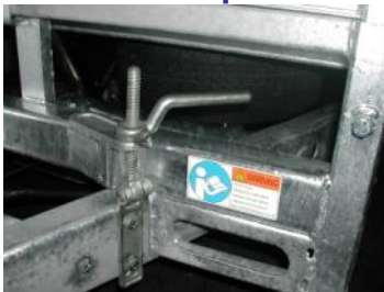
A Frame Clamp Secured
