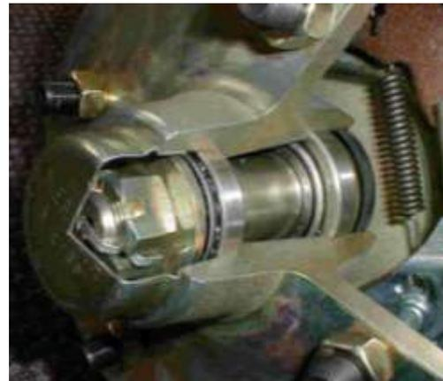
The wheel bearings are greased on assembly at the factory and should be re-greased at a minimum every 24000 miles or 2 years with axle grease 'Elf Multi 2' or equivalent.
