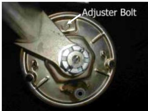
Rotate each wheel only in the forward direction of travel, whilst tightening the bolt until the wheel locks. Then, gradually back off the adjuster nut until the wheel can rotate forwards with just a slight resistance/audible brushing of the brake drum on the brake linings (This is best judged with the wheel and tyre fitted to the brake drum)
