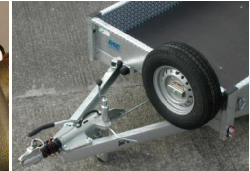
175 R 13 C 8 Tyre & Wheel Standard Spare Wheel Mounting
